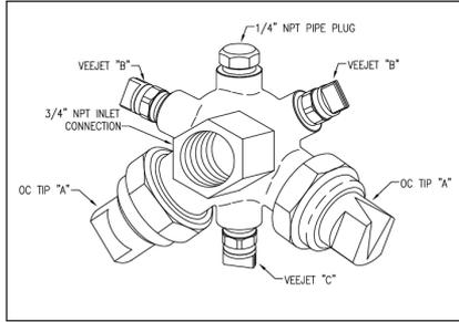
**5880-3/4-2TOC20 Boomless Nozzles With Extra-Wide Flat Spray Projection**
