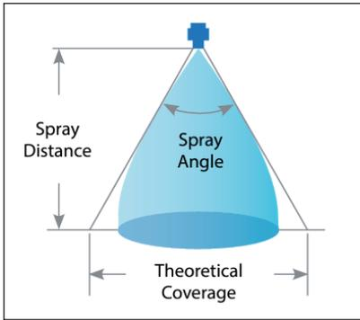
This table lists the theoretical coverage of spray patterns as calculated from the included spray angle of the spray and the distance from the nozzle orifice. These values are based on the assumption that the spray angle remains the same throughout the entire spray distance. In actual practice, the tabulated spray angle does not hold for long spray distances.
